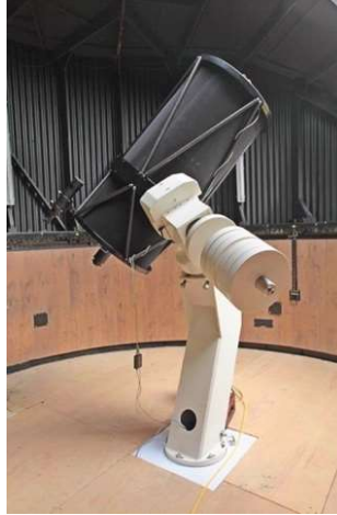
Figure 3. The 24-inch Ritchey-Chrétien telescope. Credit: Hampshire Astronomical Group.
